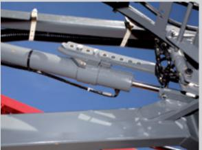
The boom height is adjusted by means of the ParaLift controlled by two rams working in traction.
