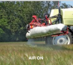
Two powerful blower units provide air to the left and right boom sides respectively. The large amount of air produced by the double fans allows for faster application speeds even under very difficult weather conditions. Each blower has an output of 2000 m<sup>3</sup>/h/m boom and a maximum air speed of 35 m/sec.
