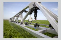
Aluminium boom structure (RHA 36 to 40 m and RA 42 to 44 m)
