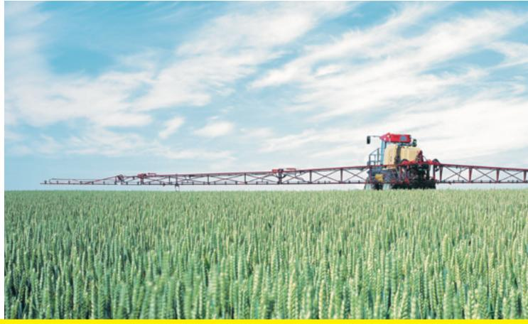
The boom has a coil spring pendulum suspension with hydraulic damping.
