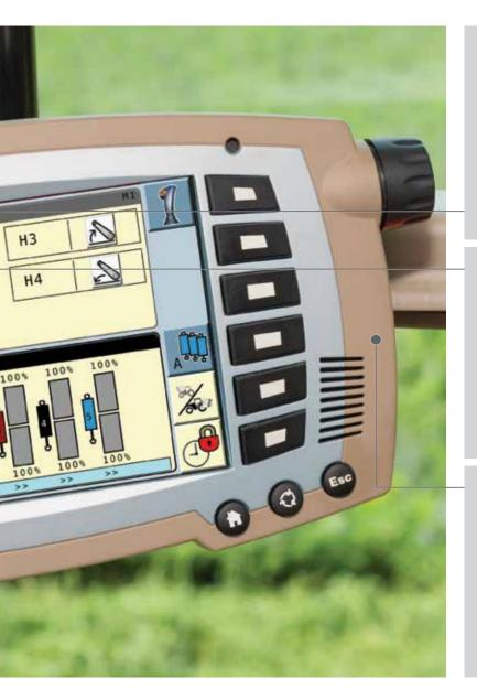
ISOBUS for total implement control – ISOBUS allows an implement manufacturer's control system to be displayed on the console screen, saving owners and operators time and money, with no need to install additional terminals in the cab. Simply plug the implement lead into the tractor's ISOBUS socket and the system automatically uploads the operating menus and displays on the screen. MF 7700 ISOBUS applies to the AEF (Agricultural Industry Electronic Foundation) certification.
