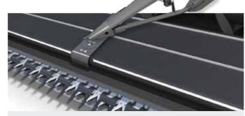
The knife is a massive 1.14m from the table auger so vision and performance are optimum. The rugged PowerFlow belts power the crop away from the knife and into the main crop elevator at a consistent speed. The belts also deflect stones rather than taking them into the machine where they might cause damage.
