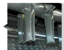
An adjustable dimple pate is standard to make sure straw is chopped consistently.
