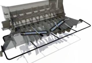
**The 6 row straw chopper** is specifically designed to give chopping and spreading performance suitable for farmers using reduced tillage operations. The knives are serrated to give a clean fine chop and reduce the power required. The fully adjustable stationary knives and straw chopper hood ensure complete control over the quality and spread of the chopped straw.
