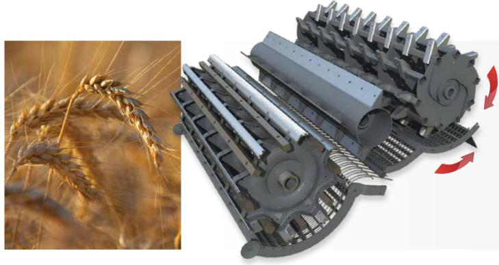
The threshing drum has added weight in the form of ballast bars which increases the inertia in the cylinder as the rasp bars threshes the heads. This reduces load on the drives, power requirement and fuel consumption.
