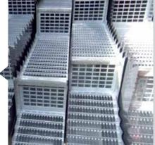
The long straw walkers feature four steps with 'active walls'. The 210 mm high, vertical sections of the walker steps are made up of permeable grids. These are the highest for any conventional combine. The front steps of the straw walkers are reinforced for maize harvestmaking the combine much more durable for variable crops
