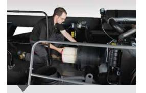
Checking and cleaning the air filter
