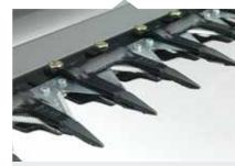
The Schumacher knife is the best performing knife in the business at 1220 cuts a minute. Self-cleaning and consistently sharp; this keeps the crop moving in tough conditions.
