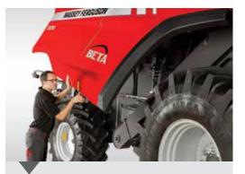
One piece panels with lights allow for quick inspection access
