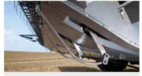
AutoLevel table control is standard with cutting height control. Smooth transition from one side to the other maintains a constant cutting height. Coupled with the Automatic reel speed feature, making table control easy on the operator.
