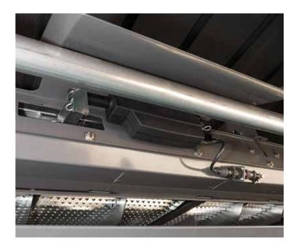
Standard electrically adjustable sieves can be altered from cab but are also part of the one-touch button combine setting system that retains information for future use.
