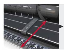
The knife is a **massive 0.9m** from the table auger so vision and performance are optimum. The rugged PowerFlow belts power the crop away from the knife and into the main crop elevator at a consistent speed. The belts also deflect stones rather than taking them into the machine where they might cause damage.
