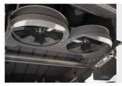
Hydraulically driven, the **chaff spreader** is fully adjustable and folds conveniently out of the way using gas struts when access to the sieves is required.
