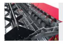
The **optional rape auger** for the PowerFlow table increases the flow of tall crops into the elevator thereby increasing the output and reducing any losses considerably. Two electrical sideknives complete the Rape auger kit.
