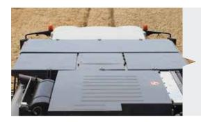
Electrical opening grain tank
