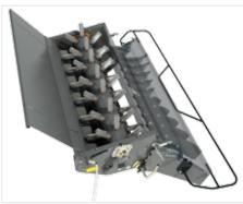
The Min-Till Chopper has eight rows of serrated blades, 108 knives and has a faster rotor speed than many standard choppers. Chopped straw length can be very short ensuring a quick breakdown of the straw which is ideal for No-Till or Min-Till cultivation systems. The chopper can achieve a spread of up to 9 metres. An additional 'dual chop' bar can be engaged easily for even more aggressive chopping action.
