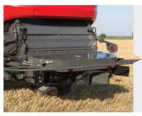
For 9m and 10.7m tables an optional **MaxiSpreader** is available which consists of two rotating impellers which propels the residue evenly over the full width. The speed of these impellers, can be controlled from the cab. If working in windy conditions, the impellers can be adjusted to compensate against any wind force by regulating the speed.
