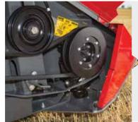
The double drive **Schumacher knife** gives a consistent speed for high output, coupled with far less stress than one drive over 10.7m for added reliability.
