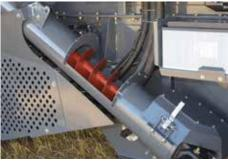
The rethresher has an easily replaceable blanking plate for rape and pulse crops for fast field turn around.
