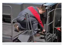
Fuel and AdBlue® fluid access is together for quick attention both have a primary filter in the neck for increased cleanliness.
