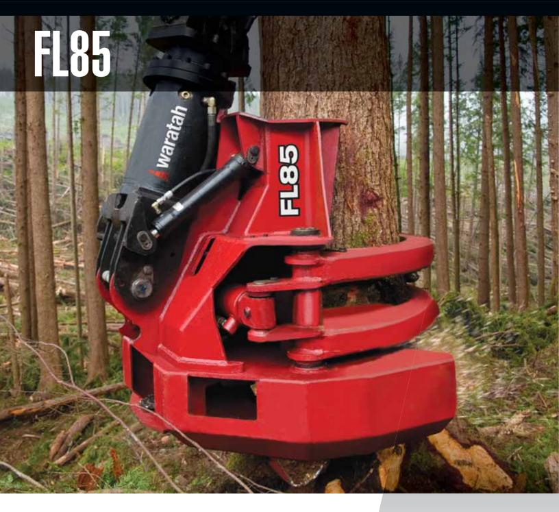
**The Waratah FL85** felling head gives you maximum versatility. It's a felling head, grapple, and saw — all in one. But this is no jack-of-all-trades, master-of-none. This well-engineered, highly productive attachment is made for major cutting and harvesting.
