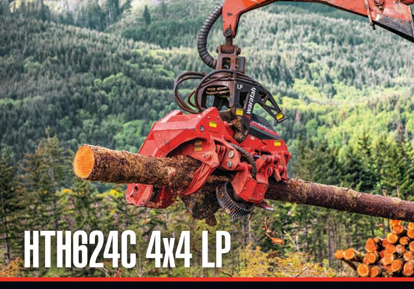
With four-wheel-drive, the versatile HTH624C 4x4 LP is built for exceptional delimbing, log handling and productivity. A shorter tilt frame permits loading trucks and improved reach for higher deck piles. Plus, the large delimb capacity allows operators to grab multiple logs clearing the yarder chute, shovel or manipulate larger single logs.
