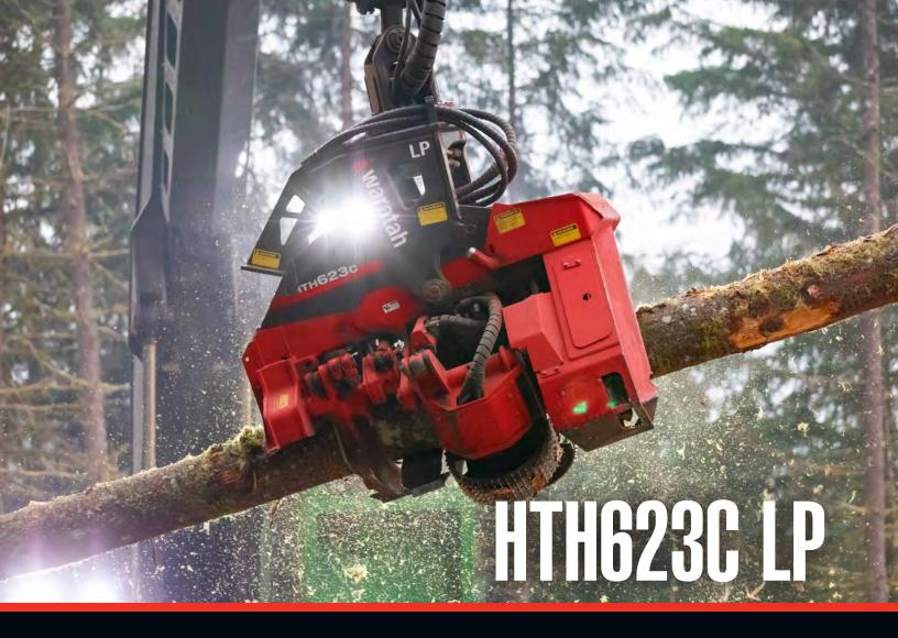
With a shorter tilt frame providing improved reach for higher deck piles, the HTH623C LP is a multi-use head built to work in tight spaces. Its large delimb opening allows for grabbing multiple logs or larger single logs, which increases efficiency and productivity for clearing the chute and loading trucks.
